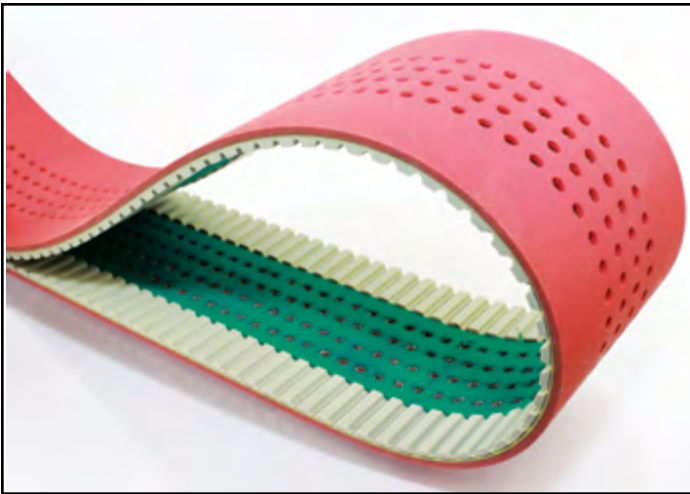
Drive side tooth removal, NFT re-insertion, hole perforations cover side
